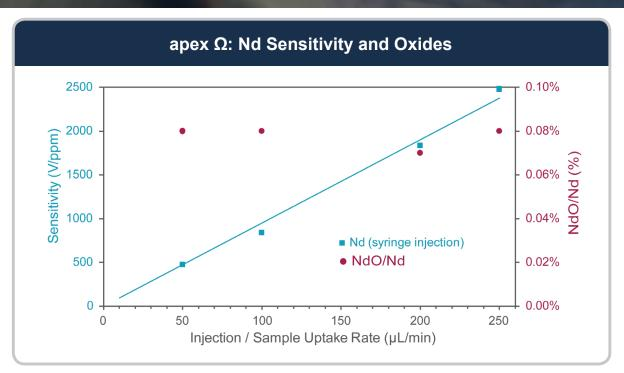
**Figure 3:** Signal increase is linear with sample injection flow rate while low oxides are maintained independent of sample flow rate.
