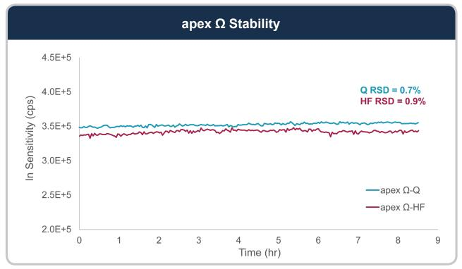
Figure 2: 8 hour stability test illustrates <  $\pm$  1% RSD (1  $\delta$ ) for both apex  $\Omega$  Q and HF.
