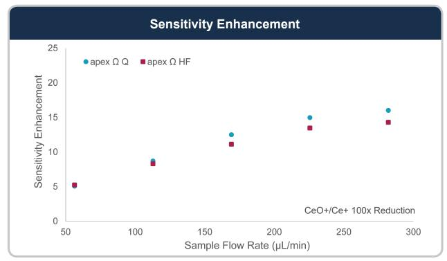
Figure 1: Similar sensitivity enhancement for both apex  $\Omega$  Q and HF.
