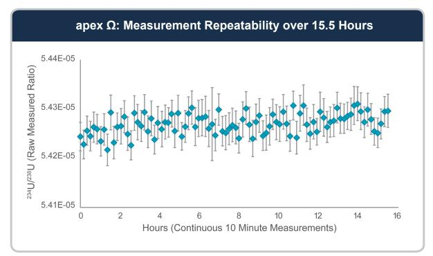
**Figure 6:**  $^{234}$ U/ $^{238}$ U measured with 131 kcps (2 mv)  $^{234}$ U on  $10^{13} \Omega$  amplifier from 25 ng/g NBS U-010. 92 x 10-minute runs spanning 15.5 hours. Raw Ratio RSD: 0.04% (external), 2se (Internal)
