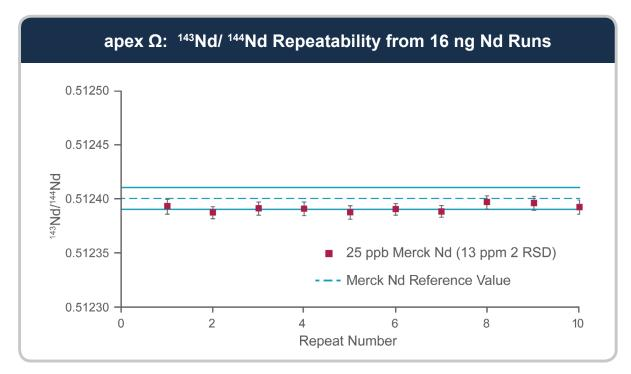
**Figure 4:** Repeatability of 16 ng Nd runs (25 ng/g solution), using apex  $\Omega$  with PFA-100 self- aspirating nebulizer and 5 minute acquisition time.
