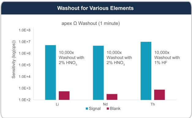
**Figure 7:** Replicate injections illustrate greater than four orders of magnitude (10,000x) washout is achieved in 1 minute for Nd. Two percent  $HNO_3$  is used to achieve 10,000x washout for Li and Nd, whereas, classic memory prone elements such as Th are washed out similarly with 1% HF.
